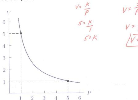
2. The volume occupied by a fixed quantity of gas such as oxygen is inversely proportional to its pressure, provided that its temperature is held constant. Suppose that a quantity of oxygen occupies a 100 liter volume at a pressure of 16 atmospheres. Write an equation for this inverse variation. If the temperature of the oxygen does not change, how many liters will it occupy if its pressure rises to 20 atmospheres? Round to 1 decimal place.
